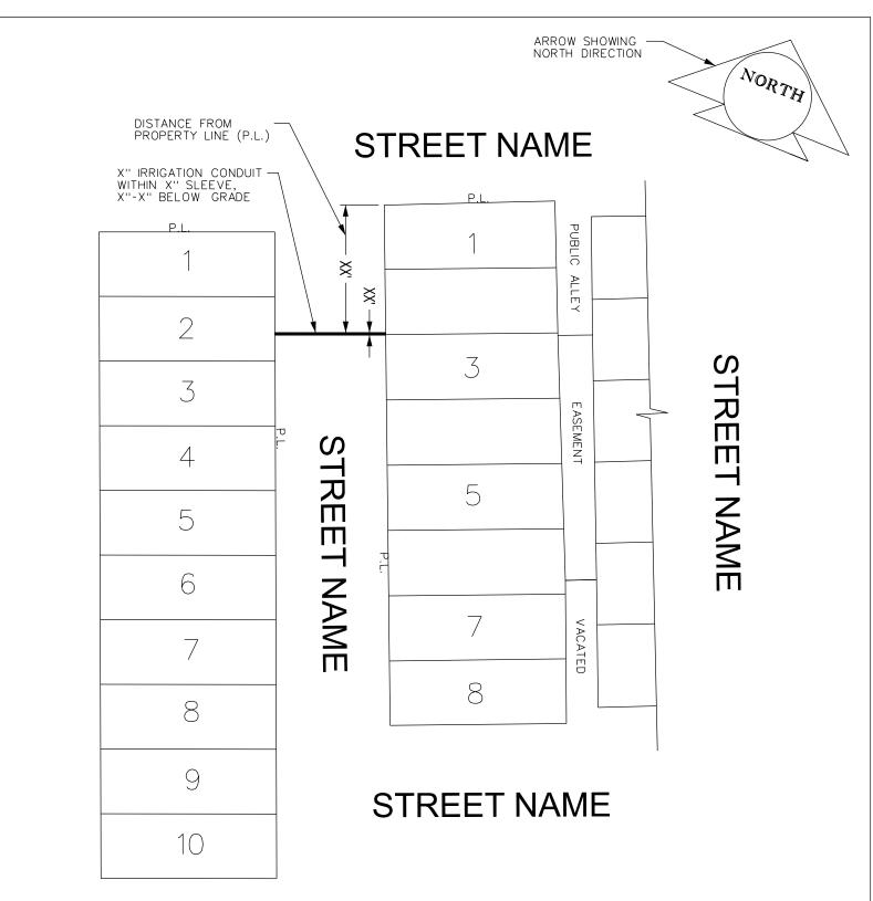
NOTE: Describe Drainage or Irrigation Line (X' Length, X' Width, X' Below Grade). Show distances from property lines and other features such as street signs, light poles, sewers, fire hydrants, etc. that are located in the proposed encroachment area.
