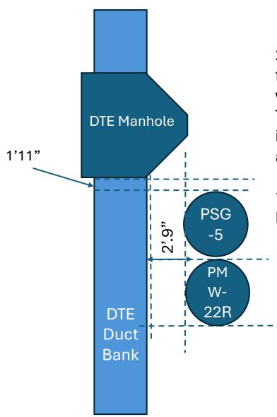
2'9" is based on measurement from east edge of DTE manhole to west edge of PMW-22R/PSG-5. The 2'9" measurement should be increased to 5' for DTE to approve.
