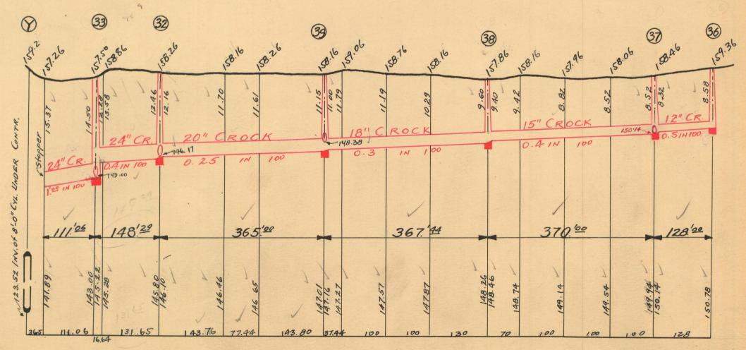
NOTE--Contractor to furnish and set as markers for all connections  $\frac{1}{2}$  inch iron rods 2 feet long with 3 inch tile collar 6 inches long.
