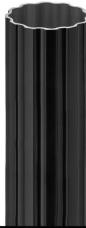
3" (Outer Diameter) Fluted Pole 0.125" Wall thickness Aluminum alloy 6063
