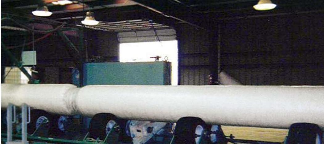
XTRU-THERM insulation prior to the application of the seamless HDPE jacket
