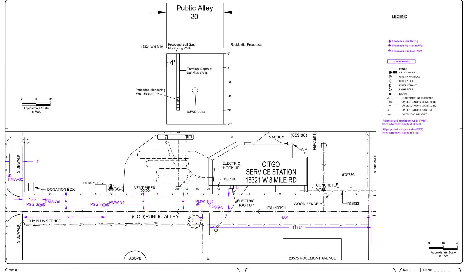
PROPSED BORING LOCATIONS IN RIGHT-OF-WAY WITH CROSS SECTION
