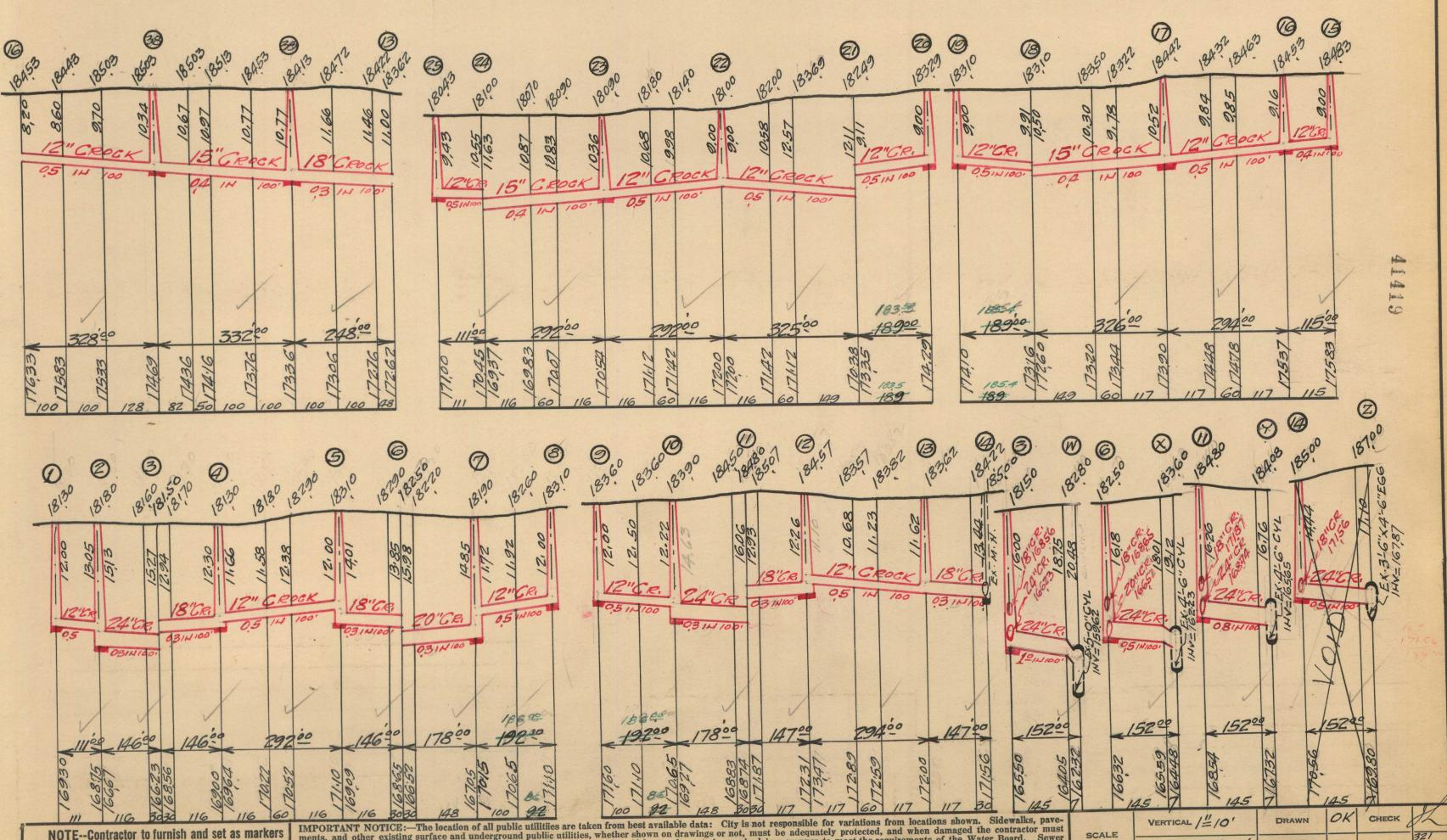
NOTE--Contractor to furnish and set as markers for all connections  $\frac{1}{2}$  inch iron rods 2 feet long with 3 inch tile collar 6 inches long.
