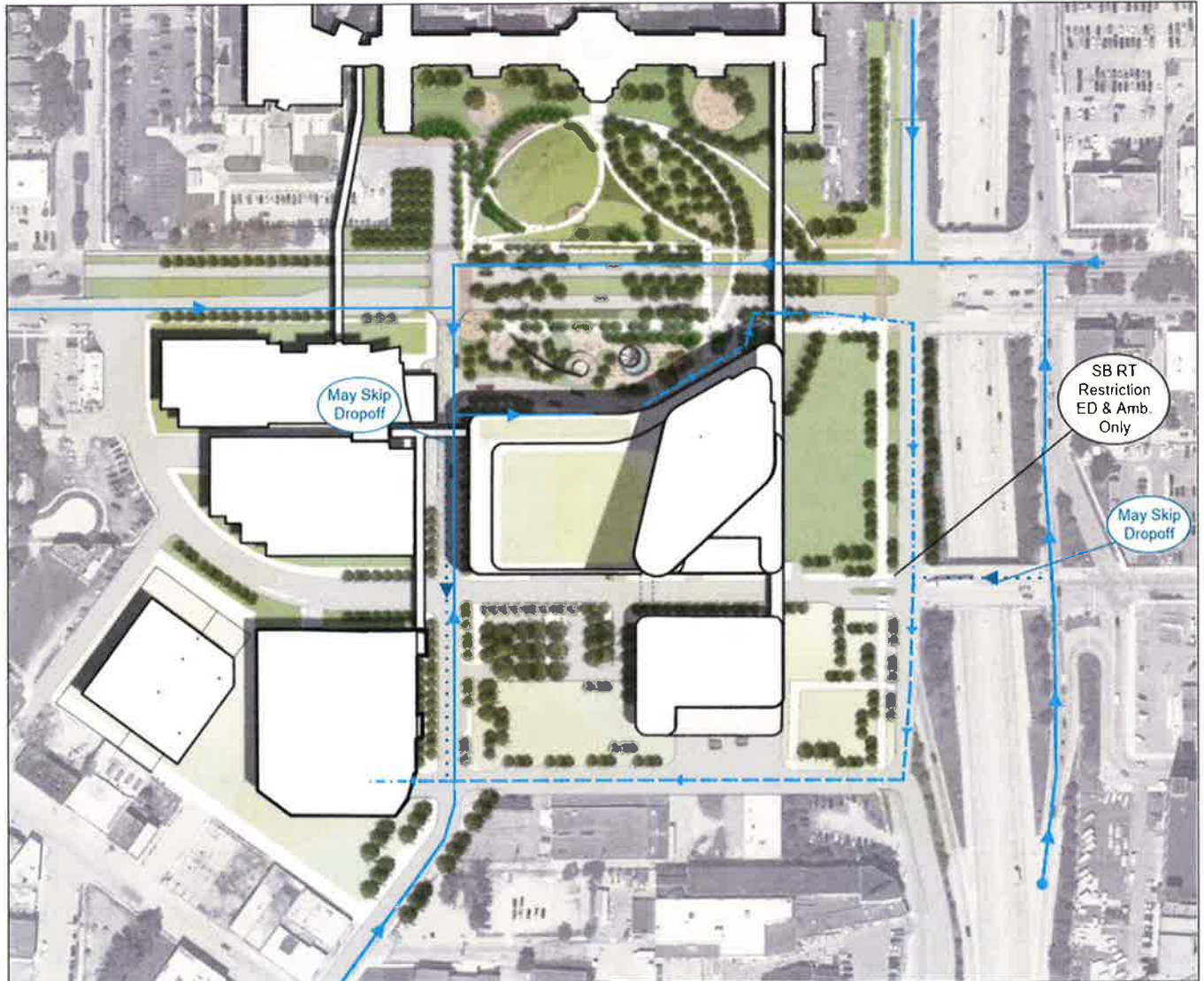
Figure 12 -- South Campus Non-Emergency Patient Site Circulation
