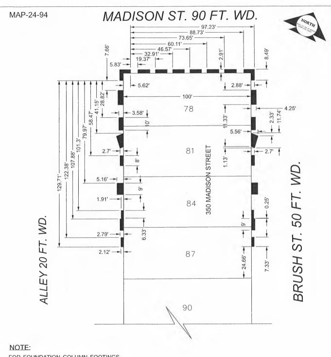
FOR FOUNDATION COLUMN FOOTINGS BOTH SIDES DIMENSIONS SHALL BE UNIFORM, UNLESS NOTED OTHERWISE.
