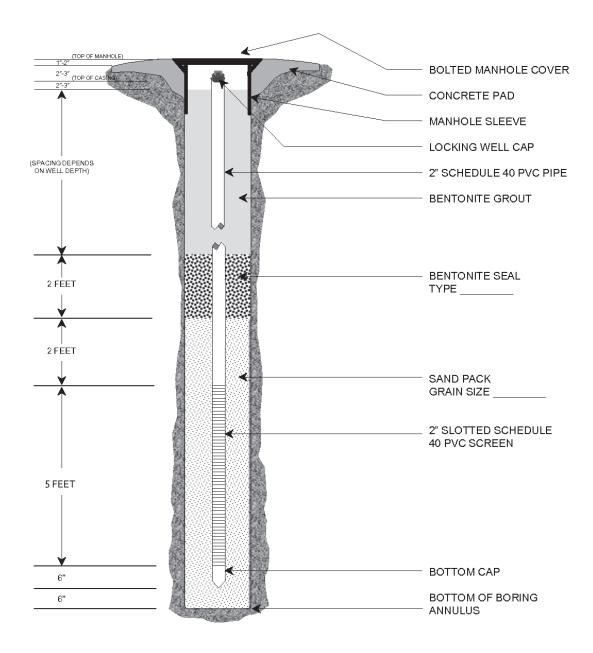
ABOVE IS AN EXAMPLE OF A TYPICAL MONITORING WELL, DEPTHS VARY DEPENDING ON THE DEPTH OF CONTAMINATION AND GROUNDWATER. MONITORING WELLS FOR THIS PROPOSED WORK WILL BE INSTALLED AT A DEPTH OF 8 FEET
