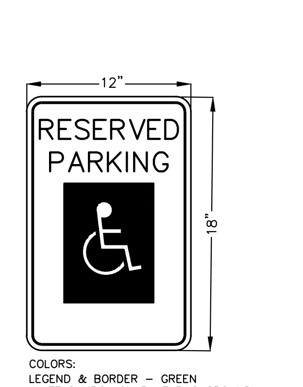
BARRIER FREE PARKING SIGN DETAIL N.T.S.
