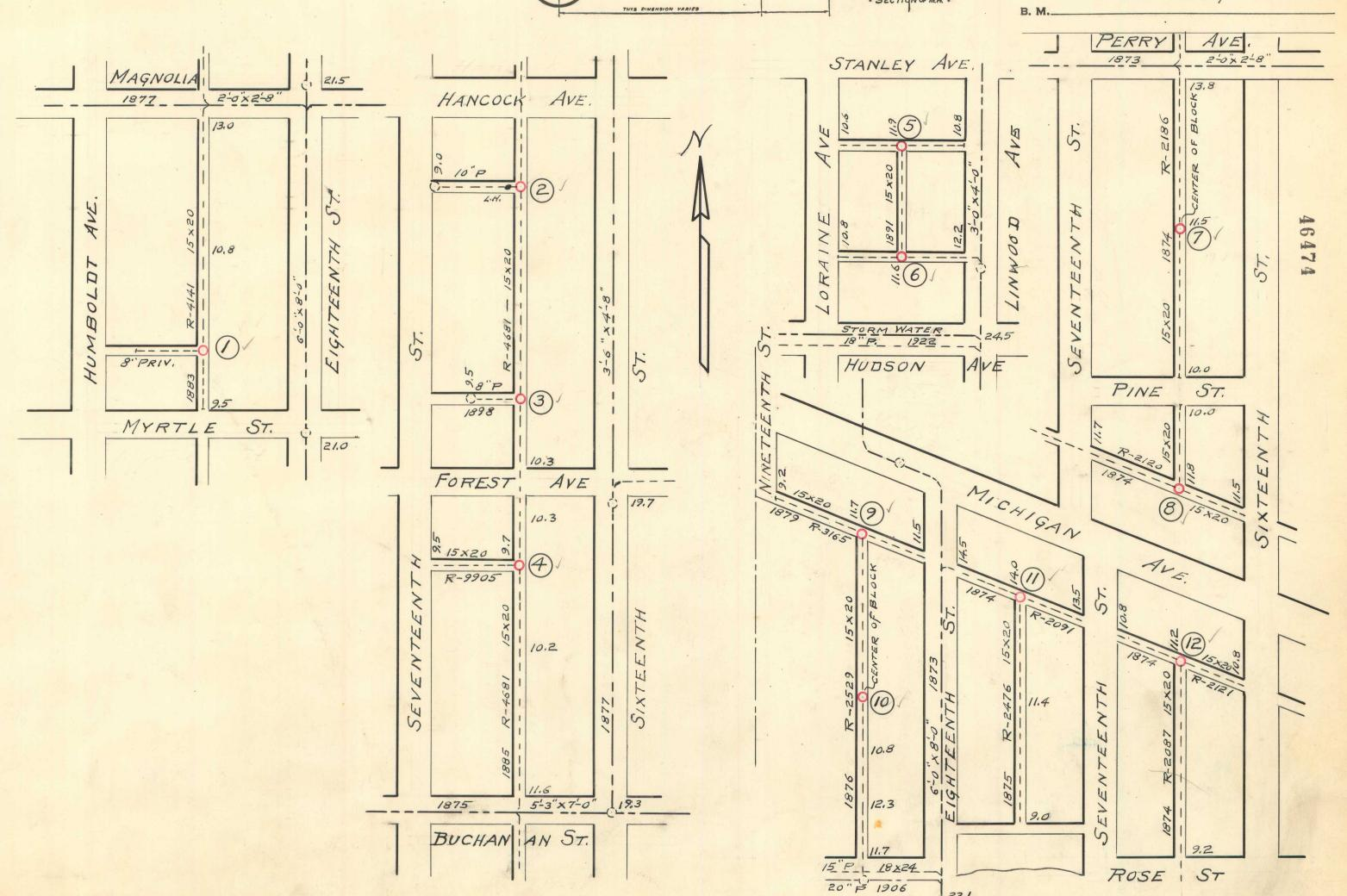
NOTE--Contractor to furnish and set as markers for all connections  $\frac{1}{2}$  inch iron rods 2 feet long with 3 inch tile collar 6 inches long.
