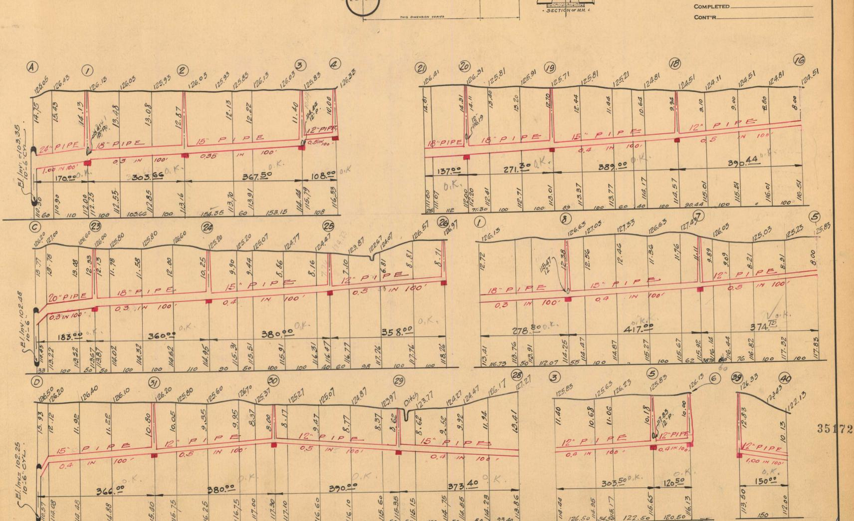
NOTE--Contractor to furnish and set as markers for all connections  $\frac{1}{2}$  inch iron rods 2 feet long with 3 inch tile collar 6 inches long.
