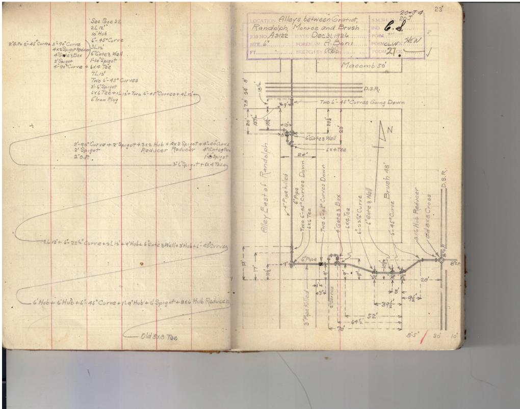
Profile of a lateral server on alley between Macomb and gratiot streets, in Block q. Brush found. A.D. 1866. 5.50 30% Scale 20 ft to an inche Harizontal. Longthe 240 feet. 4 . Certical. - Grade 10 in per 100 feet.
