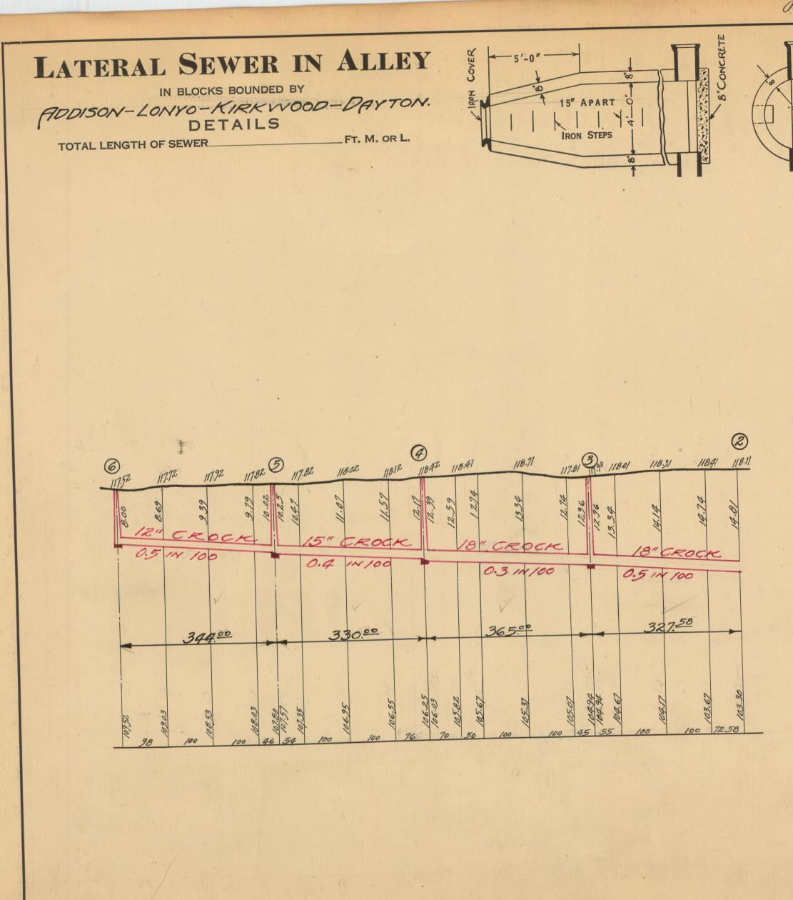
NOTE--Contractor to furnish and set as markers for all connections  $\frac{1}{2}$  inch iron rods 2 feet long with 3 inch tile collar 6 inches long.
