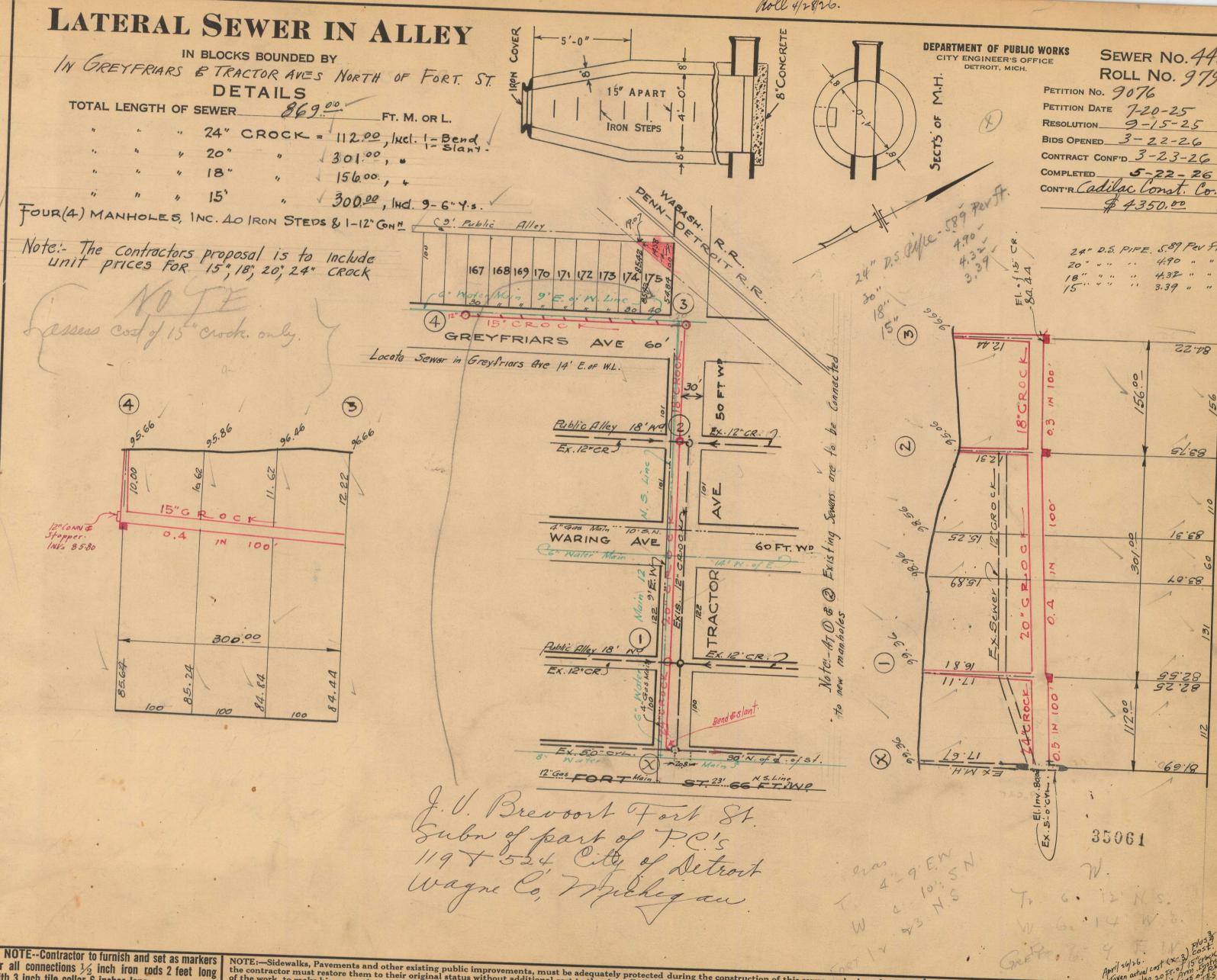
r all connections  $\frac{1}{2}$  inch iron rods 2 feet long th 3 inch tile collar 6 inches long.
