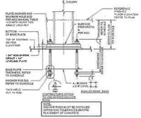
ANCHOR ROD DETAIL W/ LEVELING
