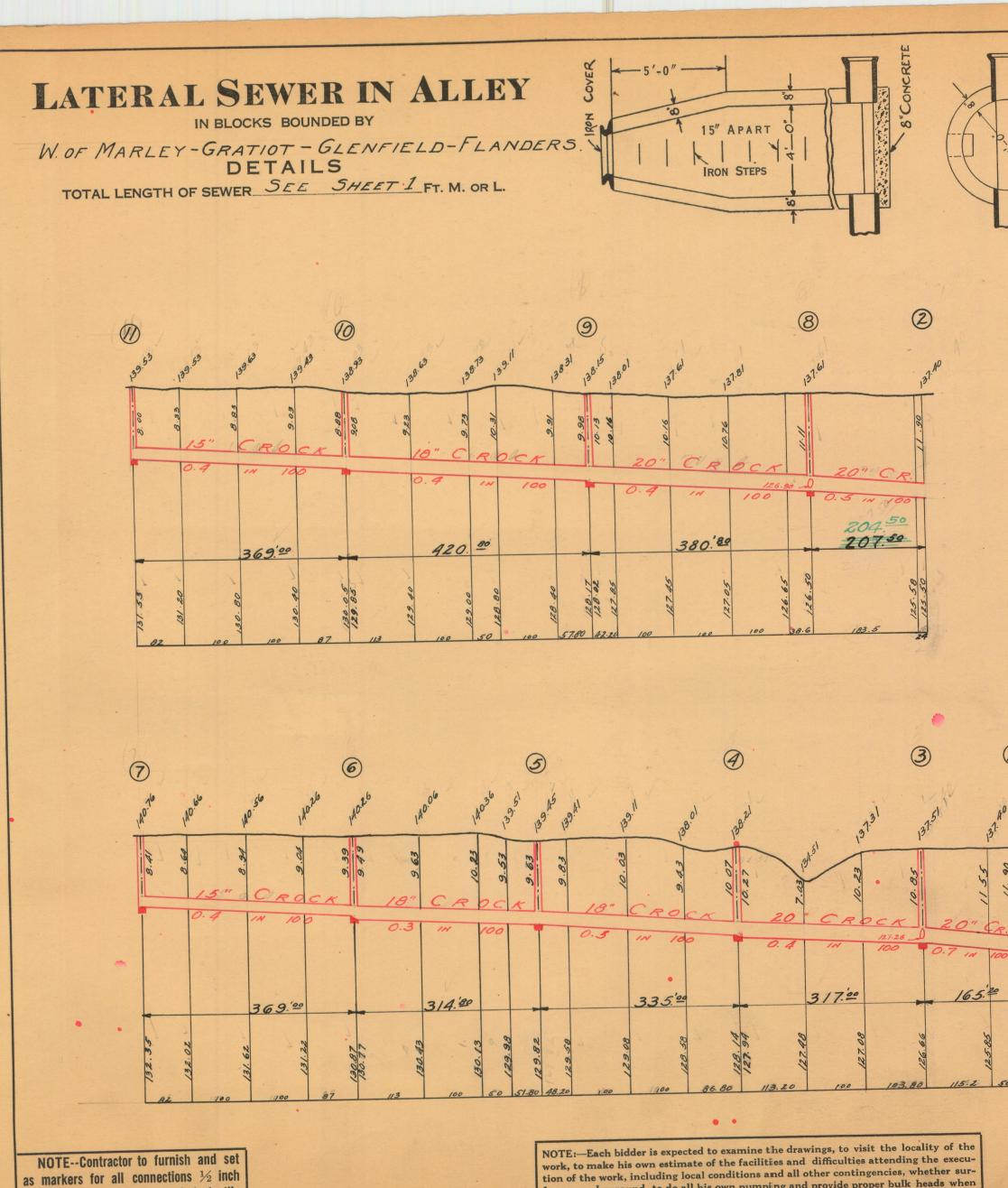
as markers for all connections  $\frac{1}{2}$  inch iron rods 2 feet long with 3 inch tile collar 6 inches long.
