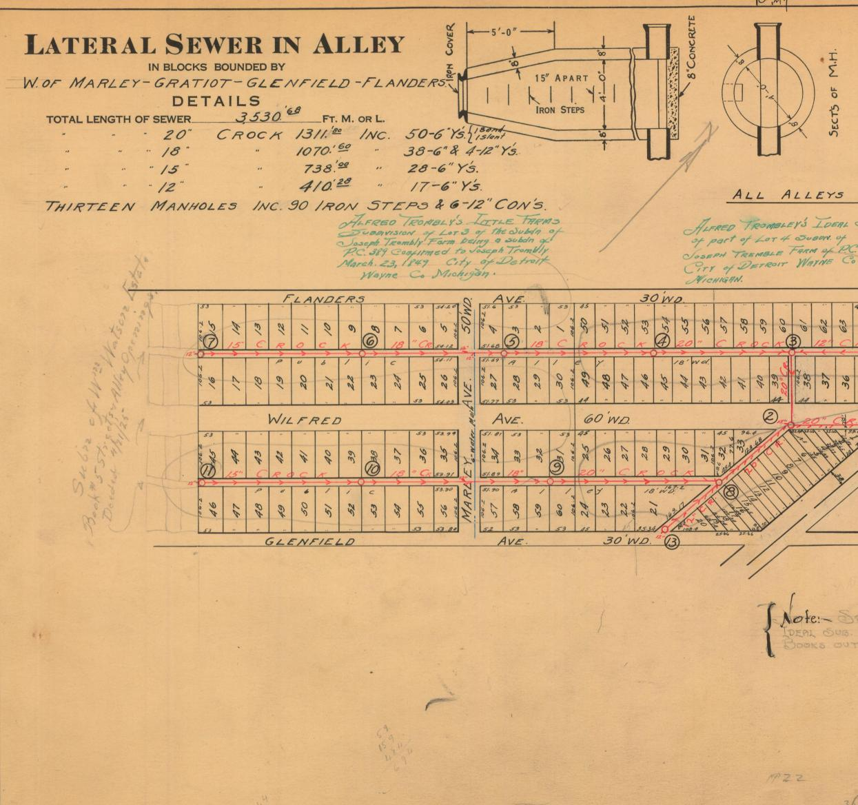
NOTE--Contractor to furnish and set as markers for all connections  $\frac{1}{2}$  inch iron rods 2 feet long with 3 inch tile collar 6 inches long.
