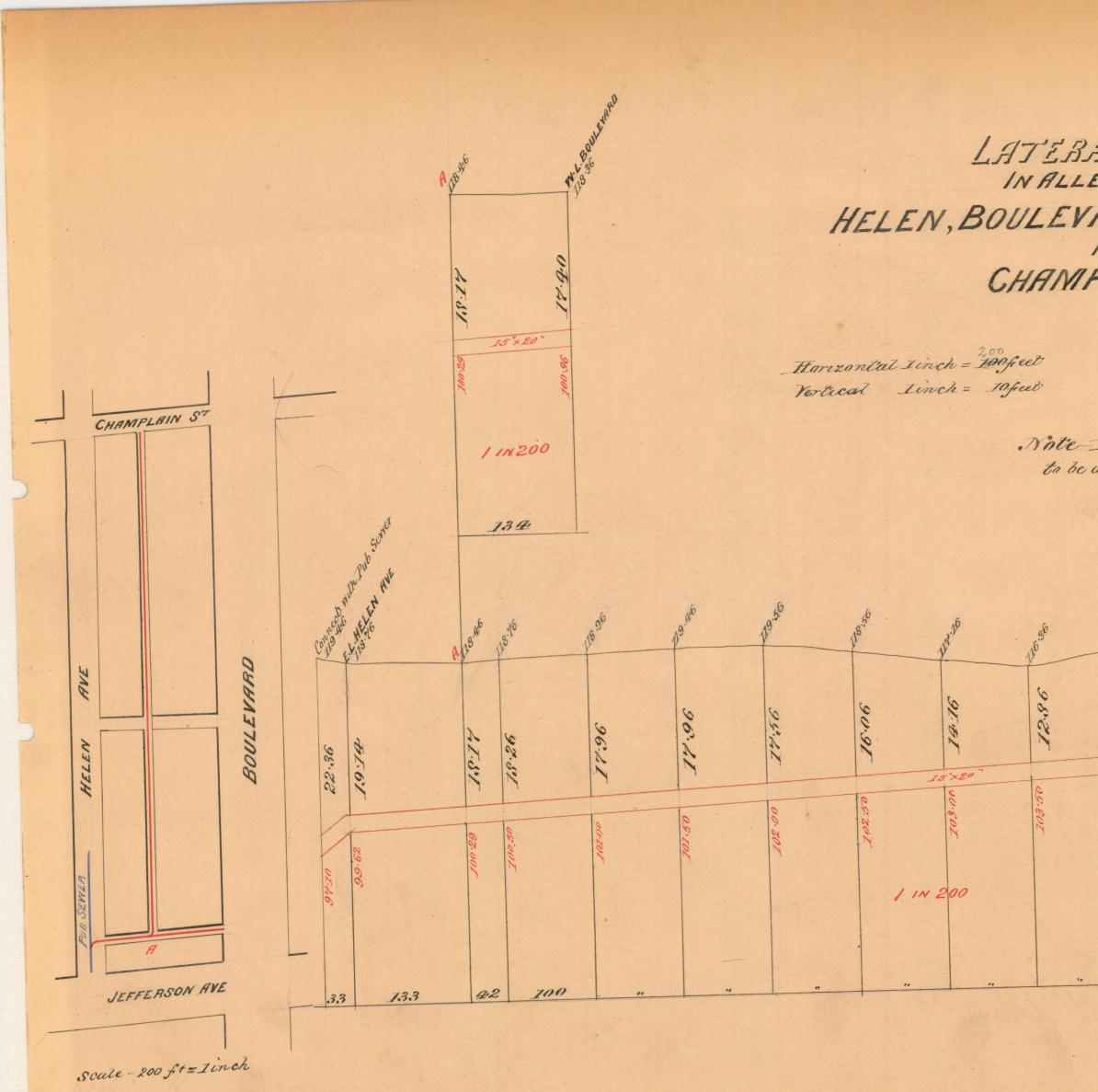
44 Sewer Nº0.9.9 Roll. Nº 177.06 John Wagner, Rate per Ft. 129 LATERAL SEYYER IN ALLEY BETWEEN HELEN, BOULEVARD, JEFFERSON, AVE AND CHAMPLAIN ST SEWER Thength, of Sewer 1452 feet Size " " 15×20-1808 Grade " " 0:50 per 100 Note-River or lake sand my to be used in mortar. 96. 2.56 200 12.86 770 10.0
