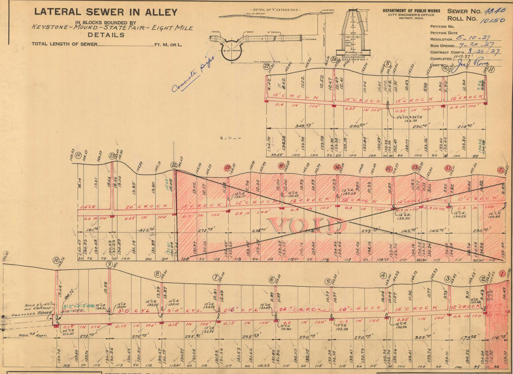
NOTE--Contractor to furnish and set as markers for all connections  $\frac{1}{2}$  inch iron rods 2 feet long with 3 inch tile collar 6 inches long.
