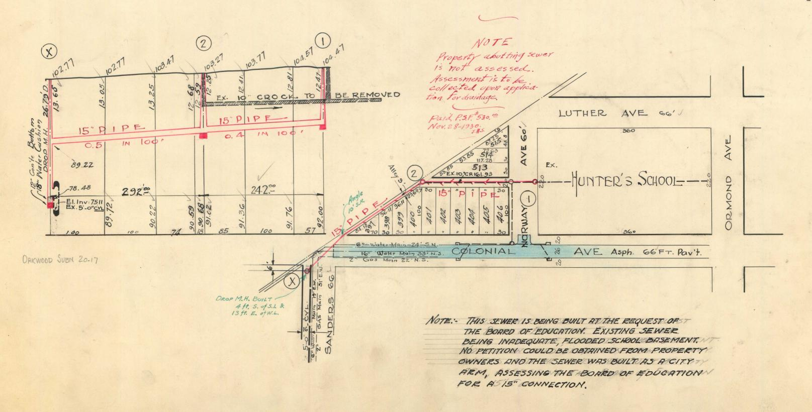
NOTE--Contractor to furnish and set as markers for all connections  $\frac{1}{2}$  inch iron rods 2 feet long with 3 inch tile collar 6 inches long.
