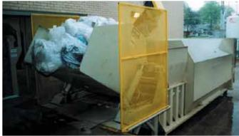
This RJ-250SC is located at a hospital and features a dock-level tipper system. Bags of waste are put directly onto the tipper and dumped into the compacter. The self-contained compactor effectively solves spillage and leakage problems associated with conventional stationary compactors and containers.
