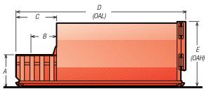
Dimensions not shown: 8' 4/%" (2543mm) Overall Width Ground Roller Widths: 61%" (1569mm) Inside Rollers 67%" (1712mm) Roller Centers 72%" (1851mm) Outside Rollers
