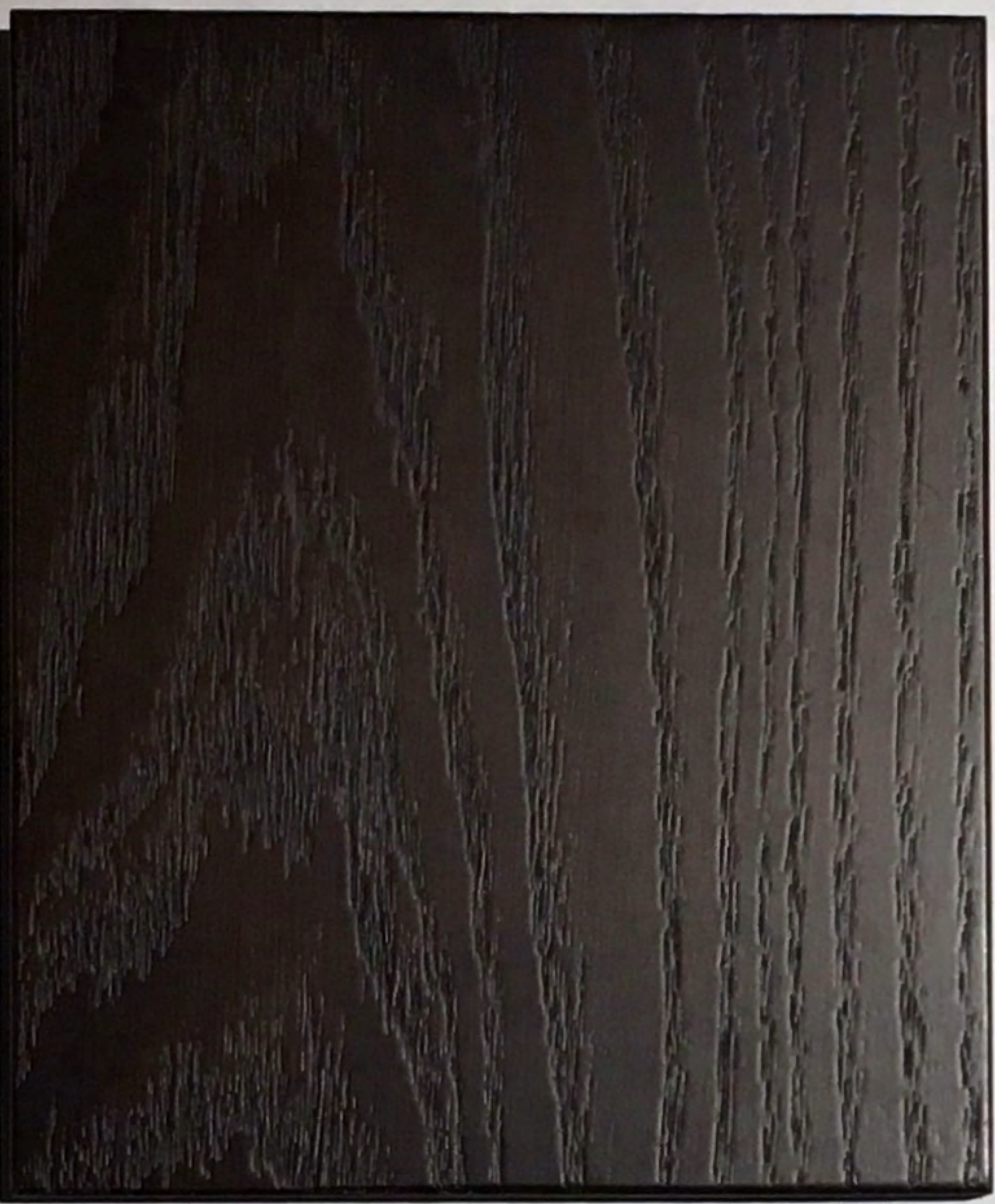
NEW AIRLOCK ENTRANCE VESTIBULE: STAINED WOOD: SHERWIN WILLIAMS "BISTRO WALNUT"
