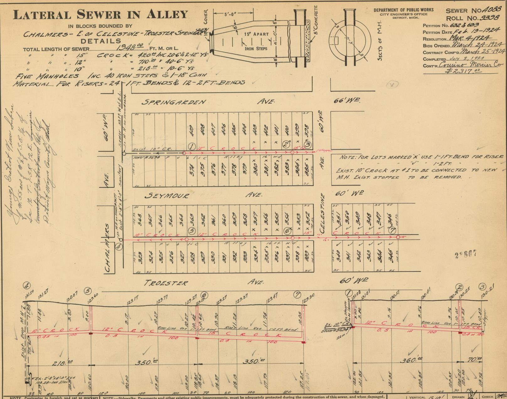
NOTE--Contractor to furnish and set as markers for all connections  $\frac{1}{2}$  inch iron rods 2 feet long with 3 inch tile collar 6 inches long.
