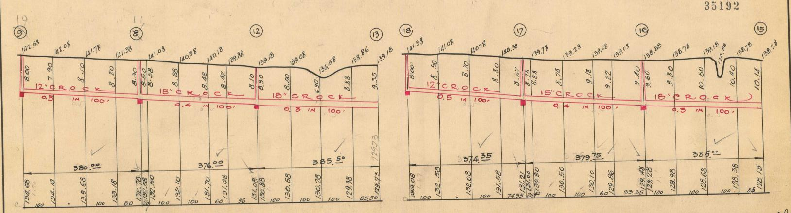
NOTE--Contractor to furnish and set as markers for all connections  $\frac{1}{2}$  inch iron rods 2 feet long with 3 inch tile collar 6 inches long.
