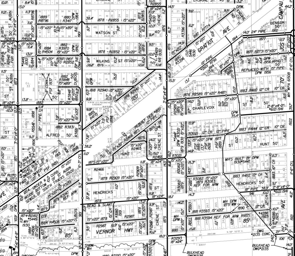
62 PROFILES OF SEWERSFOR RECEIVING BASTNS .\_\_\_ HENDRICKS WATERLOO FATTIFR ST 152 40 100 100 30 40 100 30 Measured Length of Sewer 627 Ft Measured Thenorth of Server 629 Feet SEWER Size of Server 15×20" AND 18×24" IR.CB Grade " " 0.50 per 100 Ft John Sullivan Contractor , John Sullivan Contractor - Stile of Server 15x 20" 9NO 18x 24 "IR.CB Price per Epot . 55 cts Grade " " 0.50 per 100Ft Price per Fost , 55cts ST ST ST CHENE CHENE
