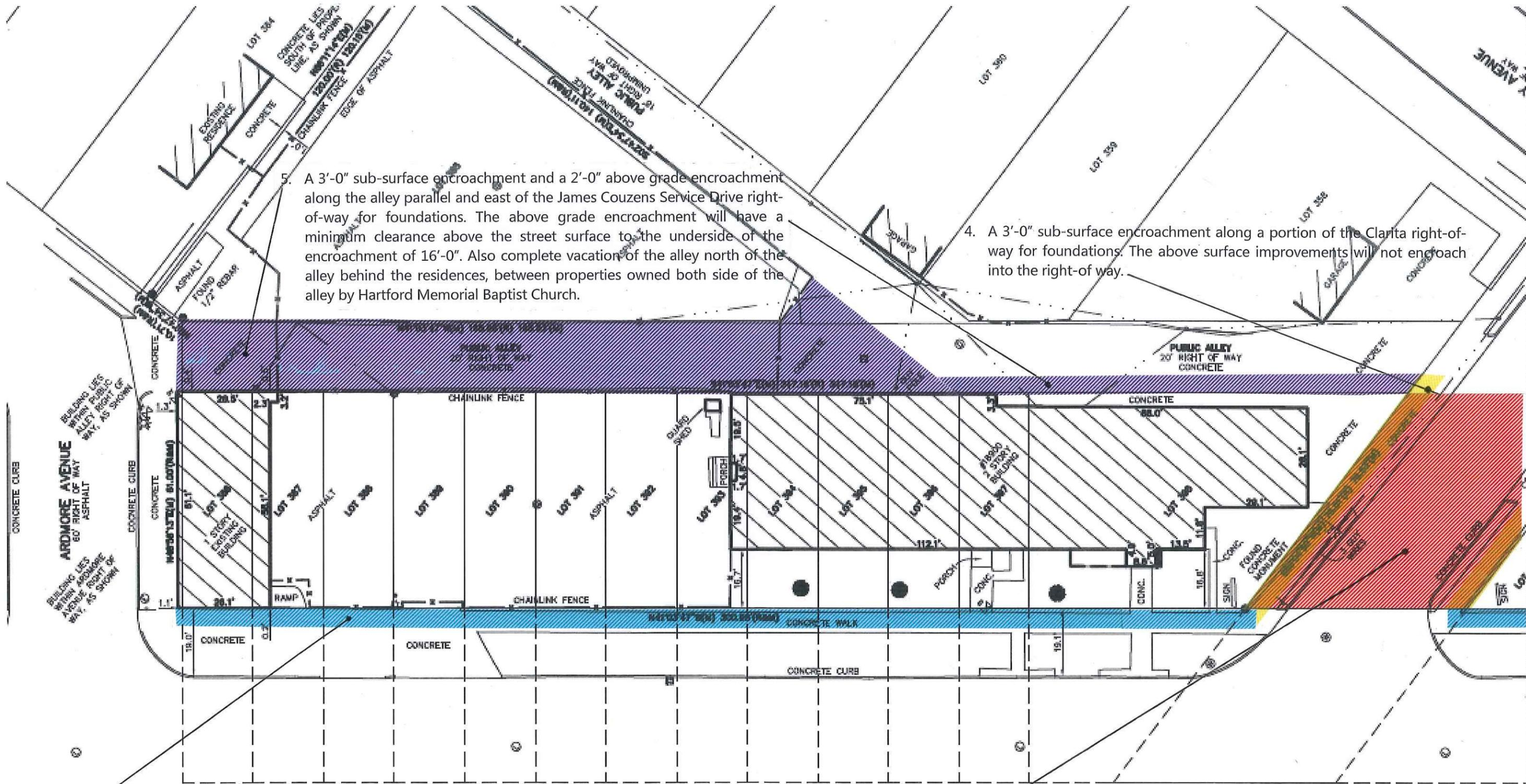
5. A 3'-0" sub-surface encroachment and a 2'-0" above grade encroachment along the alley parallel and east of the James Couzens Service Drive right-of-way for foundations. The above grade encroachment will have a minimum clearance above the street surface to the underside of the encroachment of 16'-0". Also complete vacation of the alley north of the alley behind the residences, between properties owned both side of the alley by Hartford Memorial Baptist Church.
