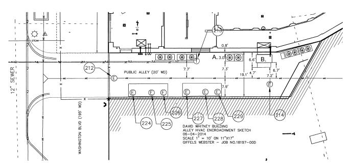
NOTE: RELOCATED AIR HANDLING UNIT (B) AND AIR CONDENSER UNIT(A).
