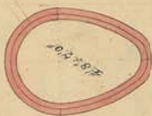
Section of Sewer - 10.35' dia.
