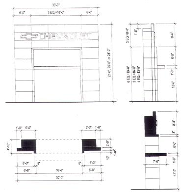
Aluminum Composite Material (ACM) Panels over 5/8" CDX Plywood and Light Gauge Metal Framing with 1/4" Typ. Joints
