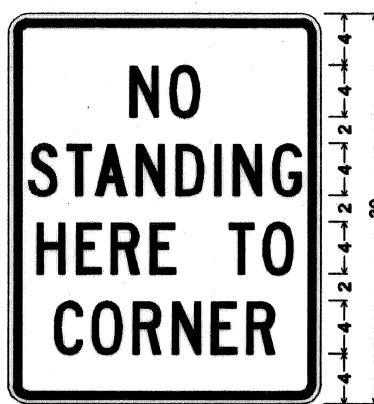
1.5" Radius, 0.6" Border, 0.4" Indent, Black on White; [NO] C; [STANDING] C; [HERE TO] C; [CORNER] C; SPECIAL DETAIL C
