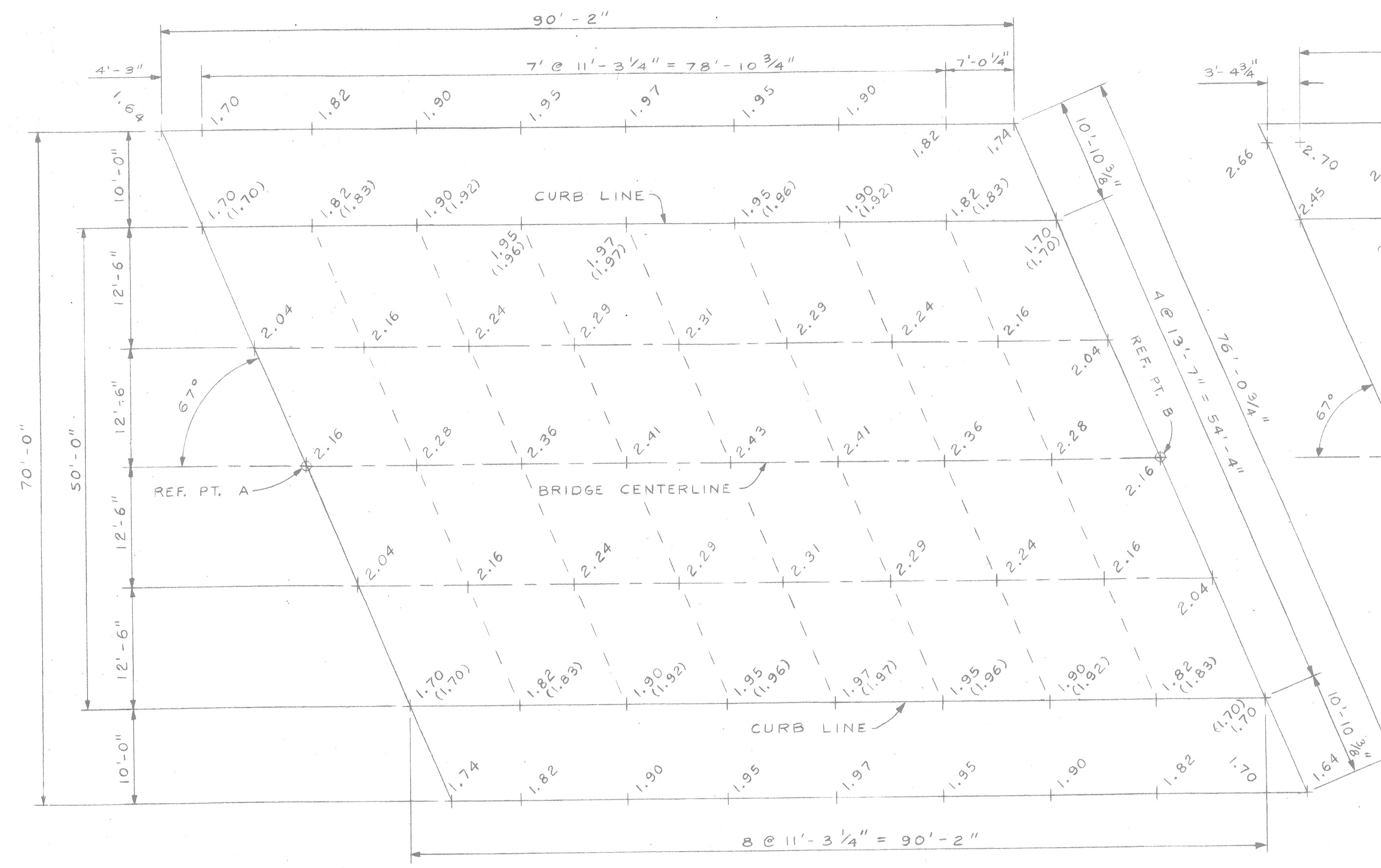
PROPOSED TOP OF DECK SLAB ELEVATIONS SCALE: 1/8" = 1'-0"
