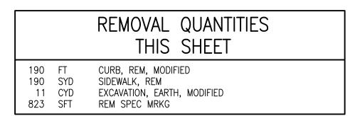
NOTES: a) CURB, REM, MODIFIED INCLUDES REMOVAL OF EXISTING PAVEMENT ADJACENT TO CURB AND HMA SURFACING OVER THE PAVEMENT.
