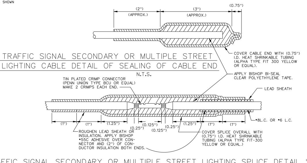
TRAFFIC SIGNAL SECONDARY OR MULTIPLE STREET LIGHTING SPLICE DETAIL "A"
